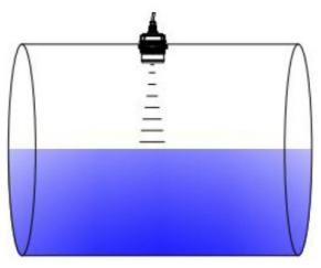
• Measurement in cylinder tanks
