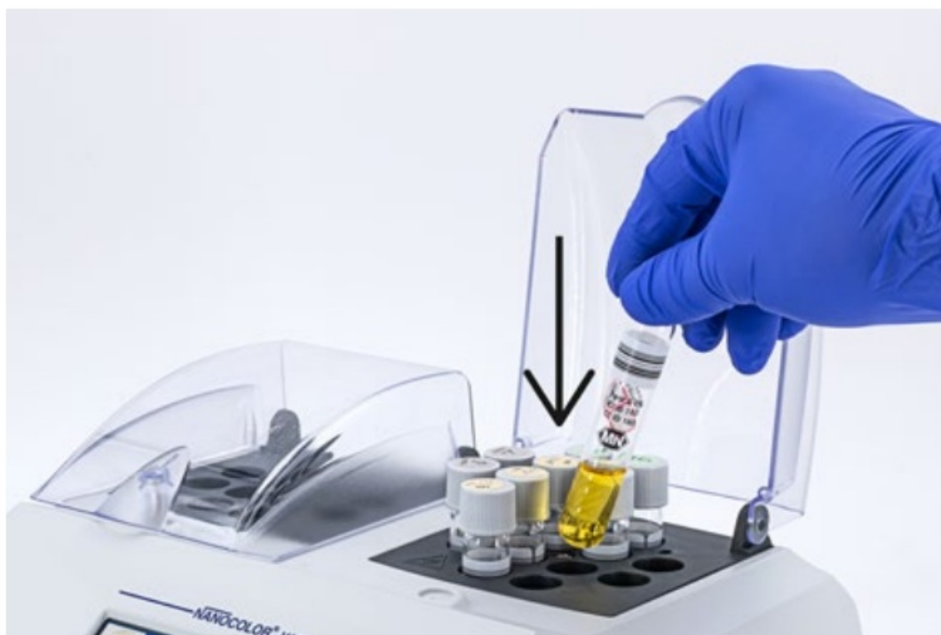
Figure 15: Inserting cuvettes into the heating block
