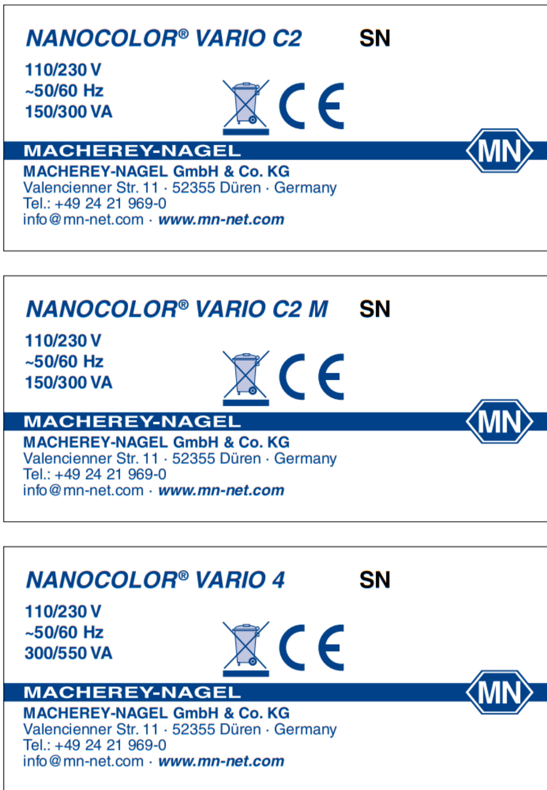
Figure 1: Type label of the heating blocks NANOCOLOR® VARIO C2, VARIO C2 M and VARIO 4
