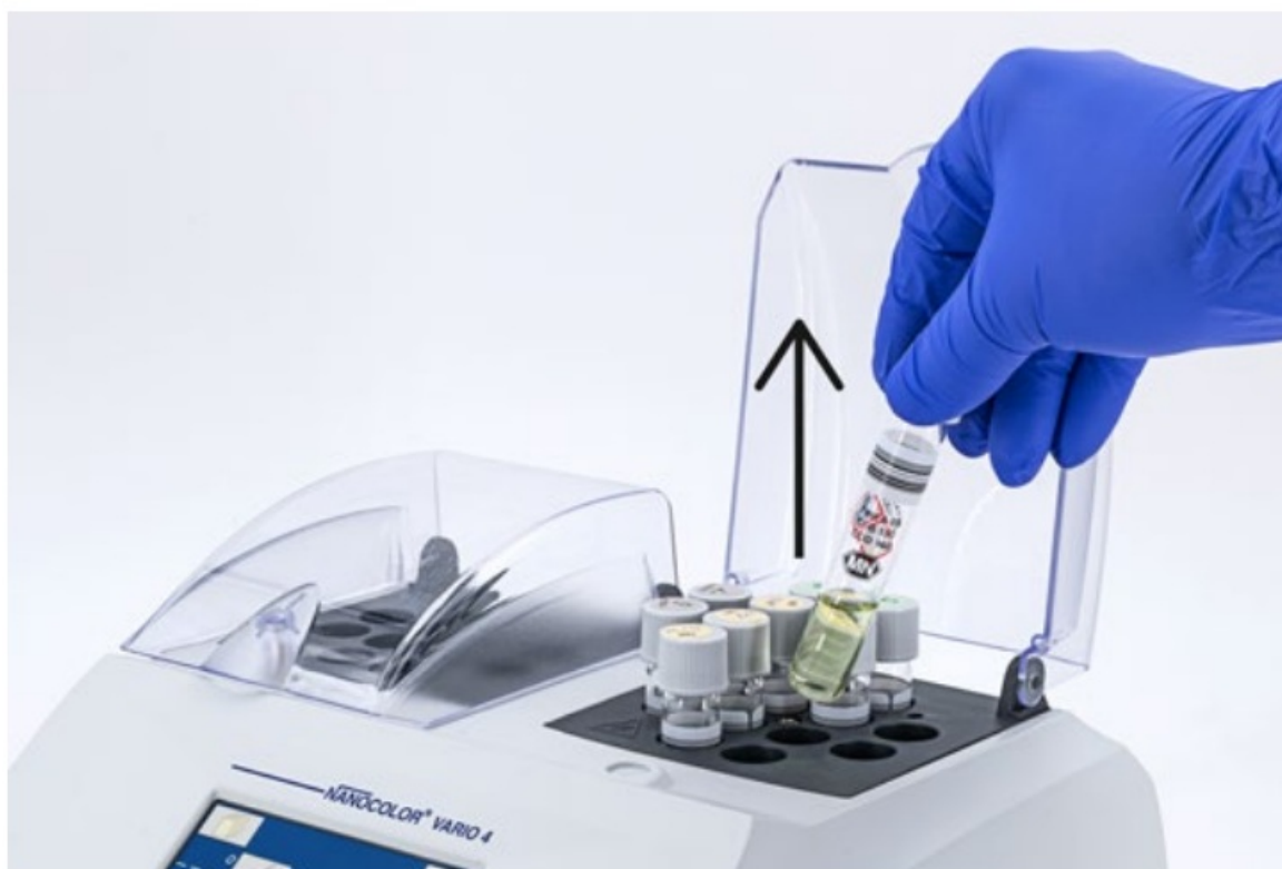
Figure 17: Removing the cuvettes from the heating block
