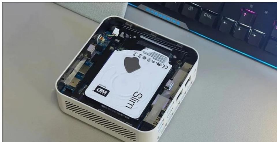
On the motherboard, you can also see a SATA cable interface, and there are screw holes on the fan bracket to fix the 2.5-inch hard drive. However, after consulting the official, we learned that Ryzen 7040 does not natively support 2.5-inch SATA hard drives and requires additional transfer lines. Therefore, Creator Mini II can only install
