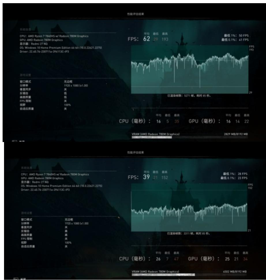
The average frame rate of “Assassin’s Creed Valhalla” in high image quality is 39FPS, which can be increased to 62FPS when adjusted to low image quality.
