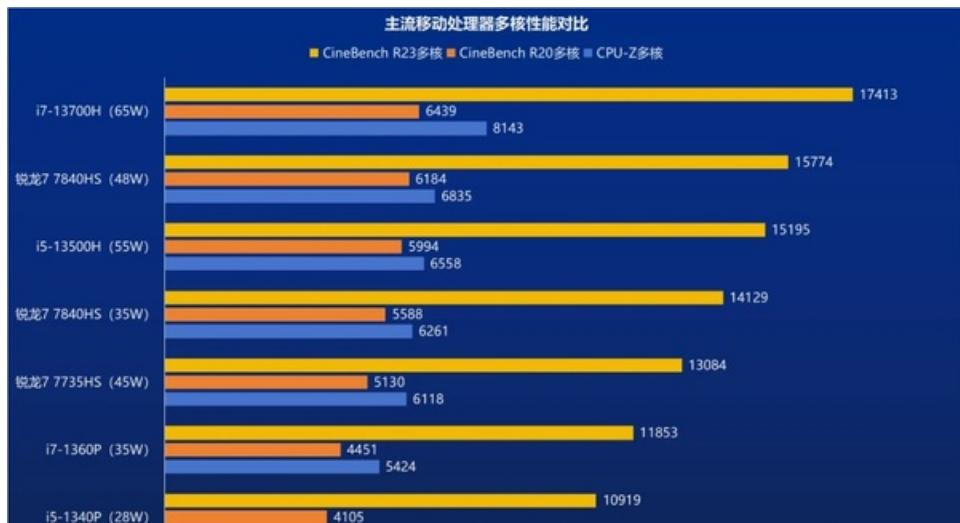
In terms of multi-core performance, the 35W 7840H is slightly inferior to the i5-13500H, but it can surpass it with 48W power consumption.
