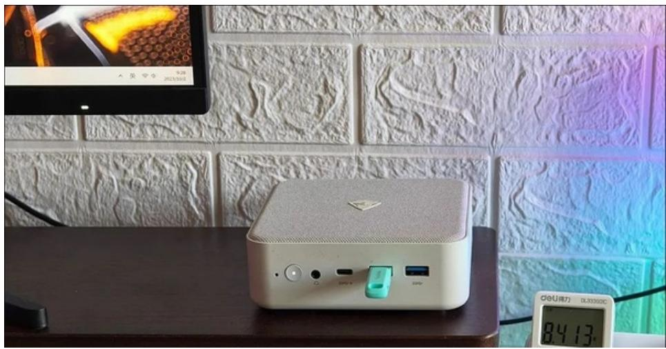
In silent mode, the FPU baking test also runs AIDA64, the processor peak value will be limited to 45W, and will soon stabilize at 35W. At this time, the CPU temperature has dropped to within 78 degrees, the main frequency is 3.4GHz, the noise value next to the host is only 44 decibels, and the power consumption of the whole machine is about 53W.
