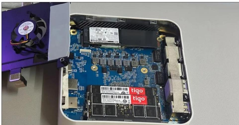
It can be seen that inside the Creator Mini II, a metal bracket equipped with a fan has been added. If you remove the bracket, you can see the memory and hard drive hidden under it.
