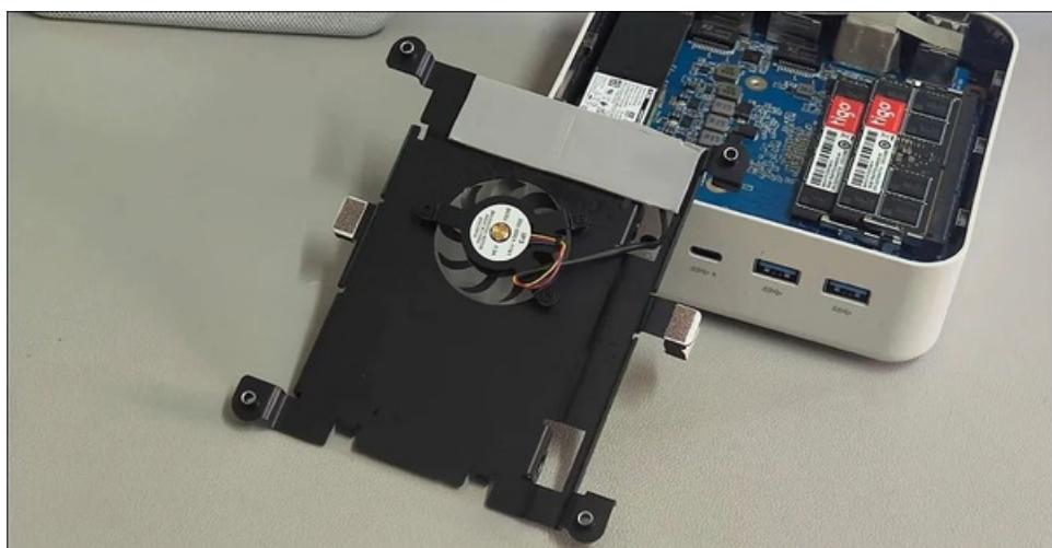
There is also thermal conductive silicone grease on the back of this metal bracket corresponding to the hard drive, which can serve as a large-area hard drive heat sink.
