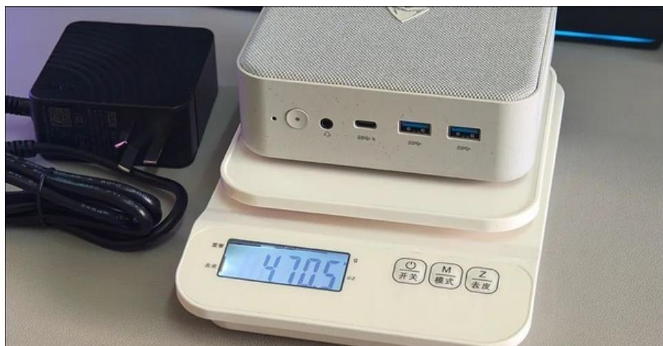
The measurements of the second-generation Creator Mini PC are similar to those of the first generation, a little narrower and a little thicker. The overall size is about 0.75L. When equipped with 2 memory and SSD as standard, the overall weight is 470g. It is a relatively mini existence.
