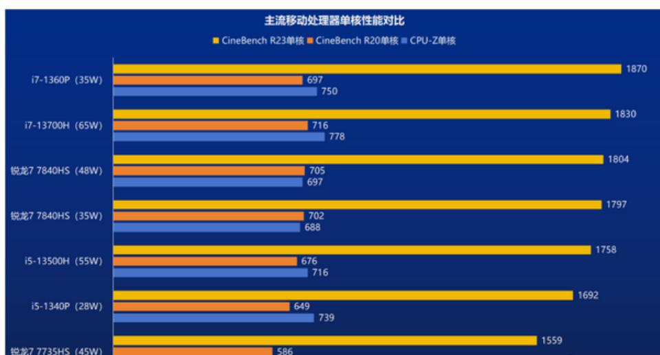
Through horizontal comparison of CPU-Z and CineBench with other common hardware platforms of Mini PCs, the single-core performance of the Ryzen 7 7840H processor at 35W power consumption exceeds that of the 55W 13th generation Core i5-13500H, and is infinitely close at 48W. 65W i7-13700H.
