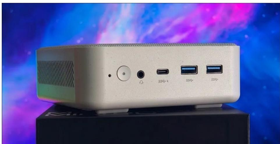
The interfaces of Creator Mini II are located on the front and rear panels. Among them, the front panel provides the reset hole, power switch, audio interface, full-featured USB4 and 2 USB-A3.2 Gen2 interfaces.
