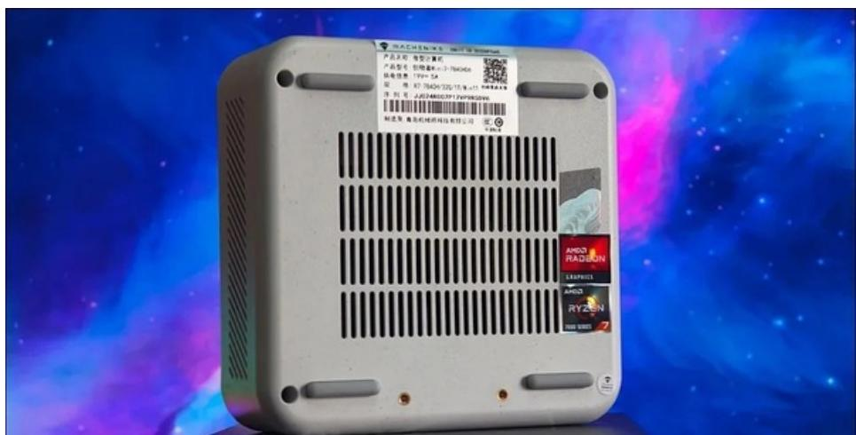
The Machenike Creator Mini 2nd-Gen has increased the air inlet area on both sides of the fuselage, and the air inlet on the bottom cover also occupies 1/2 of the area. It can be expected that its heat dissipation capacity will be greatly improved compared to the first generation.
