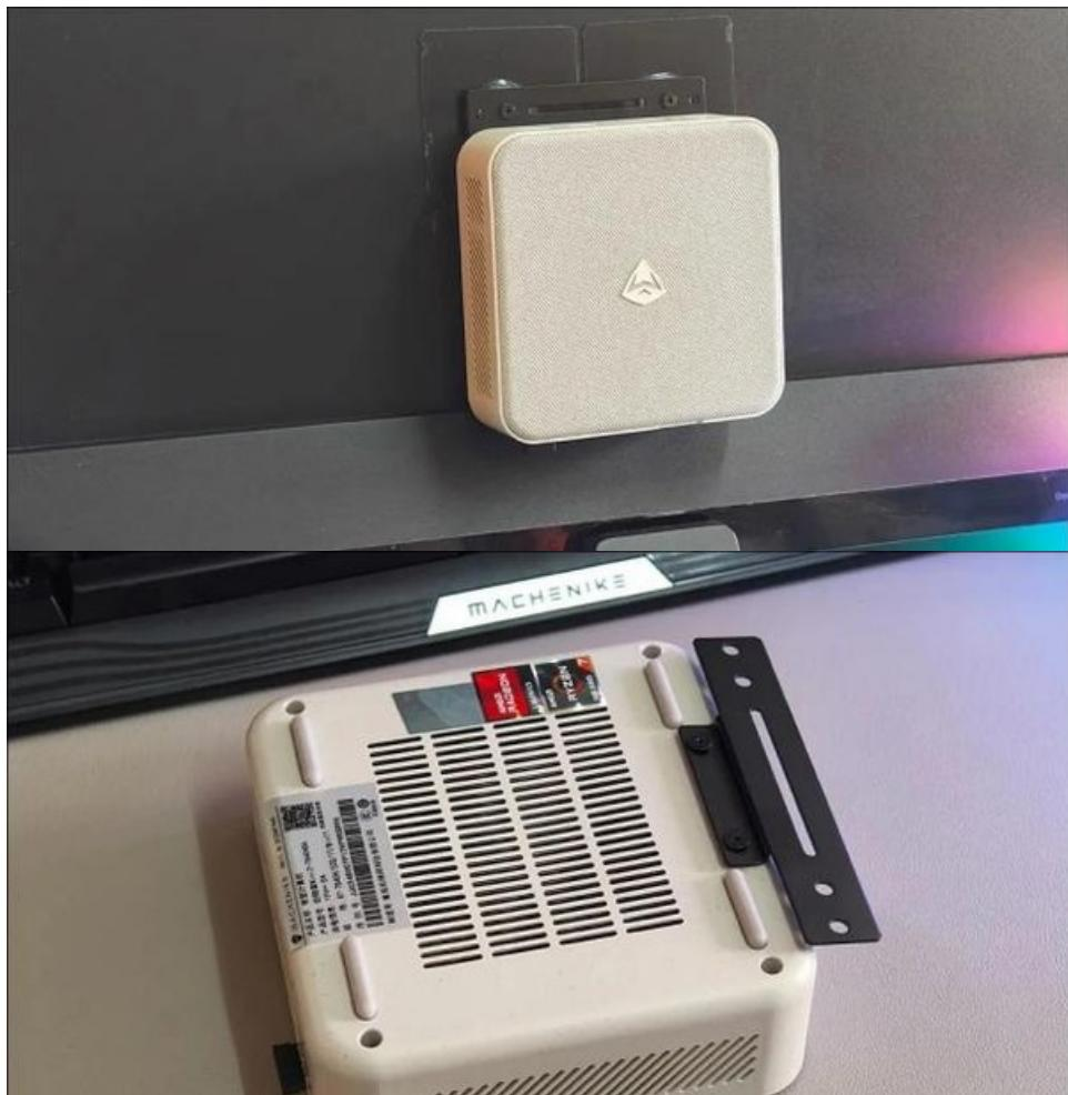
There are also screw holes reserved on the bottom cover for installing a wall-mounting bracket. With this accessory, the host can be hung on the back of a VESA-compatible monitor, further saving desktop space and turning the monitor into an [all-in-one PC].
