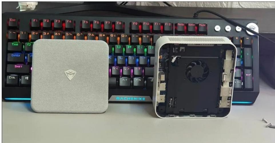
When disassembling the machine, you still need to unscrew the 4 screws at the bottom, and then turn the machine over. Through the gap on the side of the top cover, you can easily pry the cover open with your fingernails without any difficulty.
