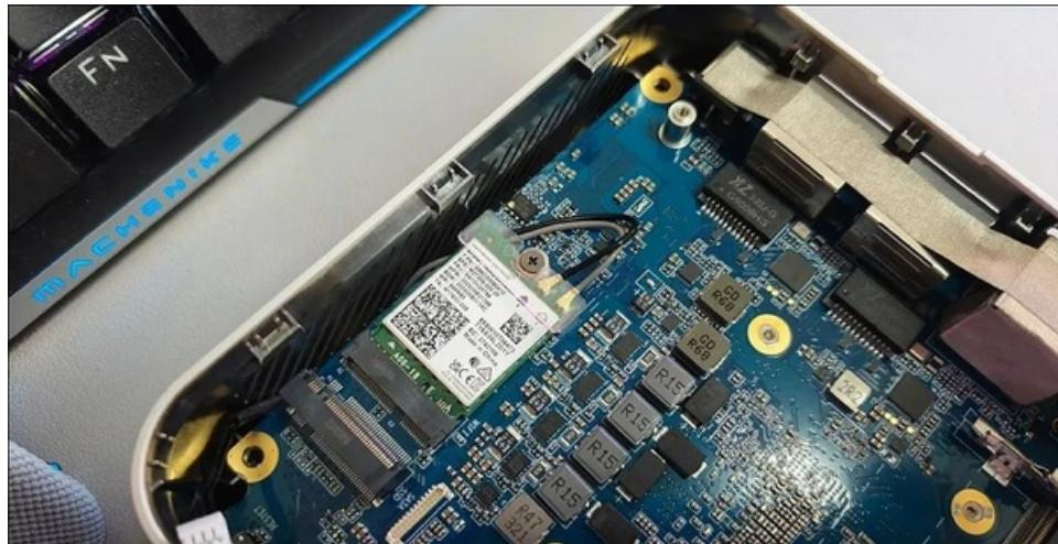
Below the hard drive is the Intel AX210 Wi-Fi 6E wireless network card, which has better performance than the RZ608 commonly used in competing products. With the help of the fan bracket, there is no need to worry about the heat dissipation problem of the network card and hard drive stack design.
