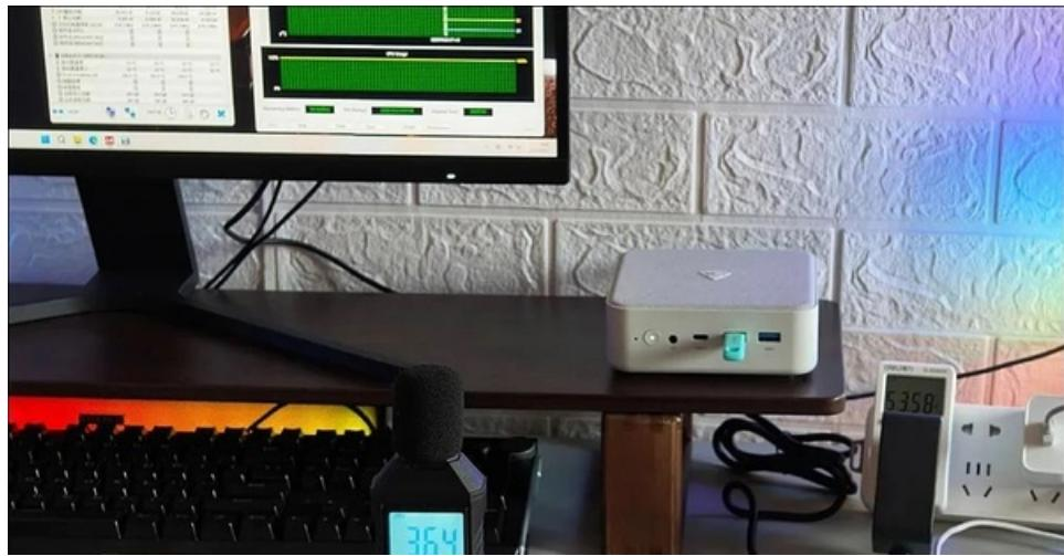
Move the sound monitor closer to the user, and the noise will be further reduced to 36 decibels, which is the same as the ambient noise and is extremely quiet. So, is there a big performance gap between the 35W quiet mode and the 48W performance mode?
