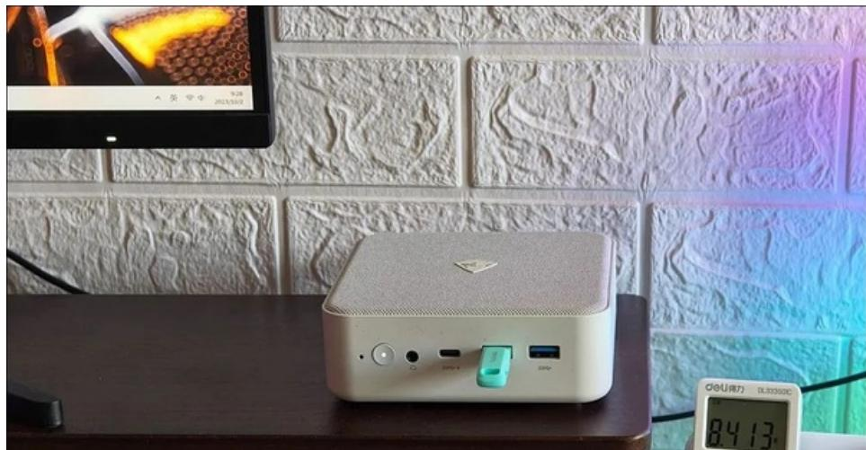
The first thing everyone is concerned about is power consumption and heat generation. In the standby state of the desktop after booting, the power consumption of the Creator Mini 2 fluctuates between 7W and 9W, which is similar to that of an entry-level Mini PC equipped with an N100 processor. It is still very power-saving.
