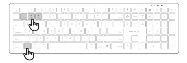
Take a look at key numbers I, 2, and 3 on the number row which are labelled BI, 82, and B3. These are the 3 Bluetooth channels that are used to pair the keyboard to your devices. To pair your keyboard to a Bluetooth-enabled device (Mac, iPad or iPhone) make sure the keyboard is on and charged, then follow the Steps below:
