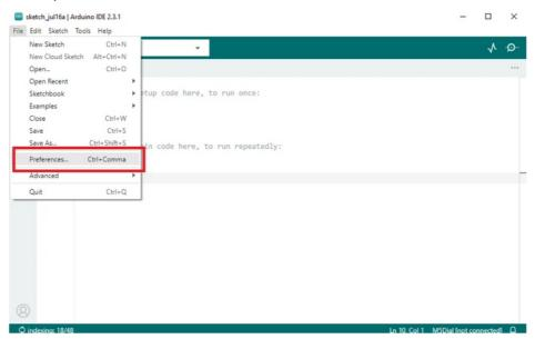
2. Copy the ESP board management URL below into the Additional Board Manager URLs: field, and save. <a href="https://espressif.github.io/arduino-esp32/package\_esp32\_dev\_index.json">https://espressif.github.io/arduino-esp32/package\_esp32\_dev\_index.json</a>
