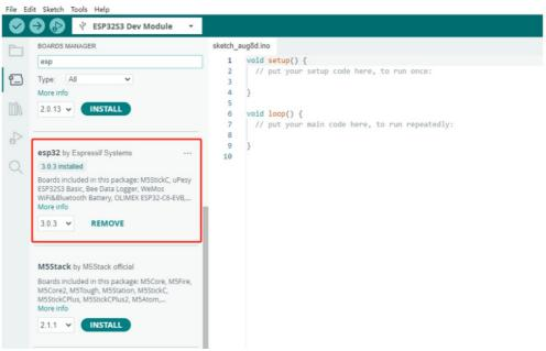
4. In the sidebar, select Board Manager, search for M5Stack, and click Install. Depending on the product used, select the corresponding development board under Tools -> Board -> M5Stack -> {ESP32S3 DEV Module board}.
