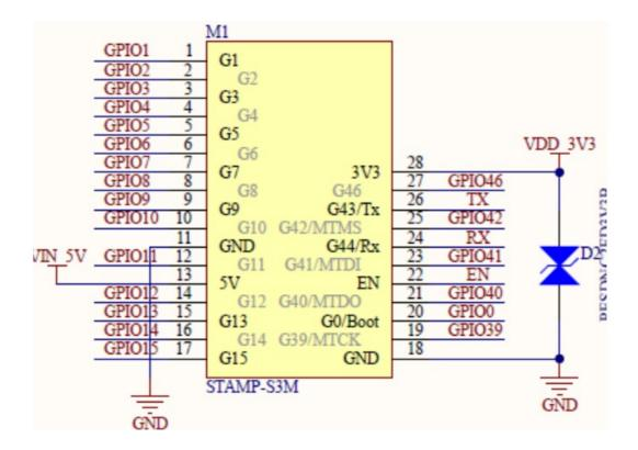
StampS3 is equipped with 28p stamp hole pad, in which pins 11 and 18 are connected to GND, and pin 13 has a voltage of 5V, which can supply power to the development board or other devices when connecting external USB. Pin 28 is 3.3V output of the development board, and other pins are GPIO interface.
