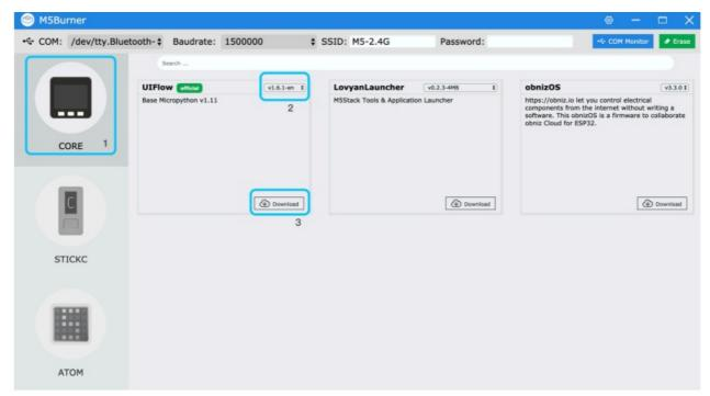
2. Then connect the M5 device to the computer through the Type-C cable, select the corresponding COM port, the baud rate can use the default configuration in M5Burner, in addition, you can also fill in the WIFI that the device will be connected to during the firmware burning stage information. After configuration, click "Burn" to start burning.
