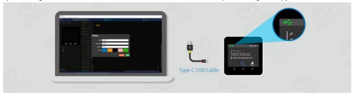
Using UIFlow Desktop IDE requires M5 device with UIFlow firmware and enter \*\* USB programming mode \*\*.
