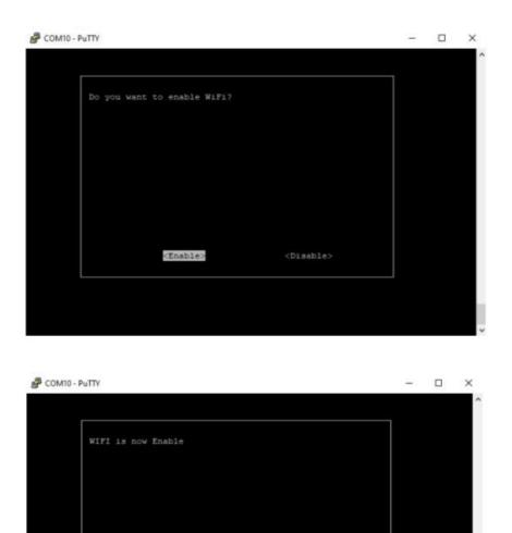
The default network configuration tool in the LLM630 Compute Kit is ntmui. You can use the nmtui tool to easily configure Wi-Fi connections.
