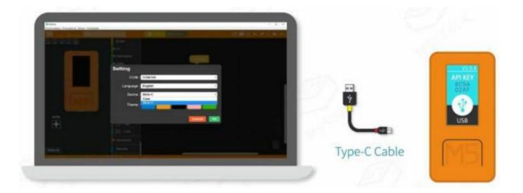
Using UIFlow Desktop IDE requires M5 device with UIFlow firmware and enter \*\* USB programming mode \*\*.
