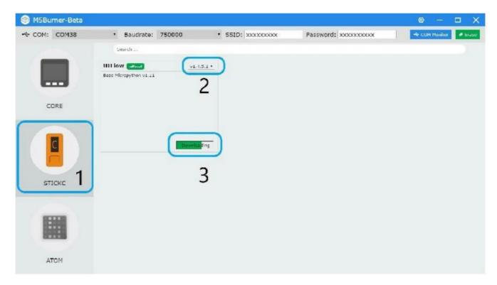
2. Then connect the M5 device to the computer through the Type-C cable, select the corresponding COM port, the baud rate can use the default configuration in M5Burner, in addition, you can also fill in the WIFI that the device will be connected to during the firmware burning stage information. After configuration, click "Burn" to start burning.
