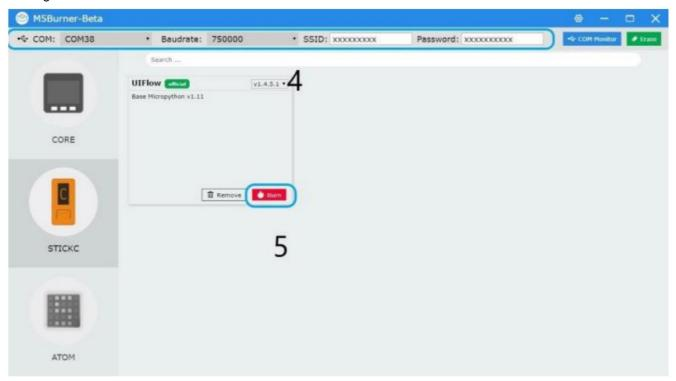
3. When the burning log prompts Burn Successfully, it means that the firmware has been burned.
