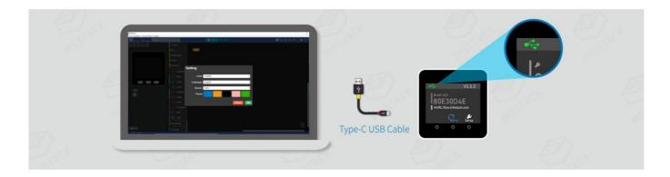
Using UIFlow Desktop IDE requires M5 device with UIFlow firmware and enter \*\* USB programming mode \*\*. Click the power button on the left side of the device to restart, after entering the menu, quickly click the right button to select USB mode.
