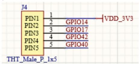
5p is equipped with a 2.54mm spacing busbar interface, and internal wiring is connected to GPI014, GPI017, GPI042, GPI040, and 3.3V.
