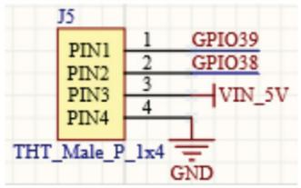
The 4p is configured with 2.54mm spacing bus ports, and the internal cables are GPI038, GPI039, SV, and GND.
