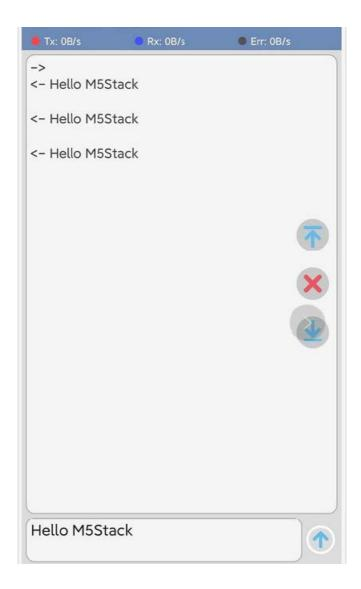
After the debugging tool sends a message, the device will receive the message and print it to the serial port.
