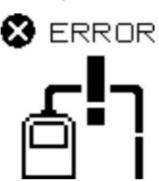
• Low Voltage Error, Check the battery.
