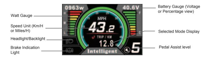
**Note:** For the battery gauge, voltage view is recommended as it provides a more accurate battery capacity.
