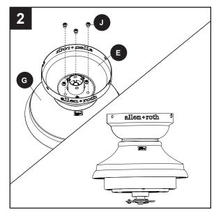
3. Raise the fan and place the canopy (E) on the hook of the mounting bracket (D), temporally leaving hands free for the wiring process. Then, place the receiver from the remote pack (Z) inside the mounting bracket (D) with the flat side facing the ceiling.
