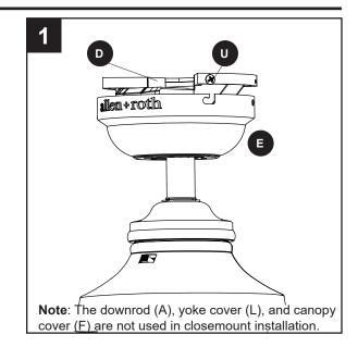
2. Secure the canopy (E) with the mounting bracket screws (U) previously removed (Step 4, page 8). Tighten all mounting bracket screws (U) securely.
