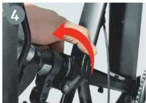
Finally, lock the lever. The seats should not be able to move with the lever in the closed position.
