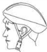
Incorrect Forehead exposed
