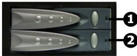
Figure 11 Hard disk drives status and activity status LEDs - model 4040
