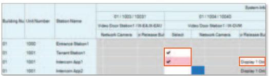
If a mobile app needs to interact with an IXG-DM7 entrance station that is using both relays, set the value to display 2 in order to have both door release sliders show up on the mobile app.
