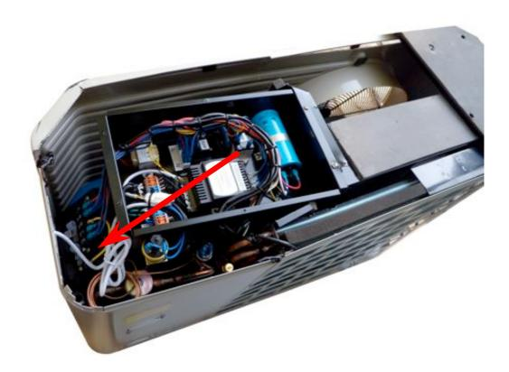
Remark – For models with 3 phases, switching 2 phases may cause an inversion in the rotational direction of electrical motors, which could damage the unit. Therefore, a protection device has been built in, which will interrupt the circuit if the connection has not been performed correctly. If you see a red LED light up at the top of this protection device, **2 phase wires have to be switched**.
