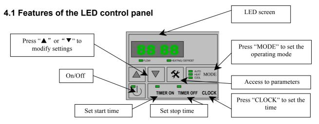
With the "On/Off" key "\( \bullet \)", the heat pump is turned on or turned off (stand-by status). If the LED next to this key lights up, the heat pump is turned ON.
