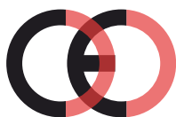
False CE Mark (too close)
