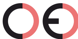
False CE Mark (too far)
