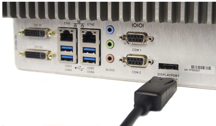
Figure 5 Single DisplayPort Connection
