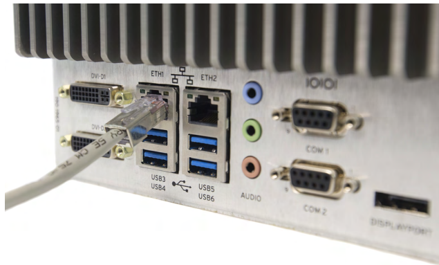
Figure 8 Ethernet Network Connection
