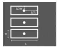
Drill four holes (Depth: around 60 mm; Diameter: around 8 mm) into the road.
