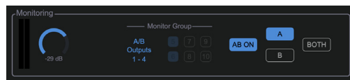
Figure 6-6: When A/B Mode is enabled, the Monitor Group controls both pairs of A and B outputs (Main Out 1-2 and Line Out 3-4, respectively). See "A/B Mode" below.
