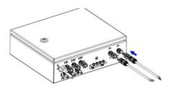
10. Cover each power cable connector with a plastic sleeve.
