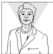
Fig. 4: Microphone pickup angle.
