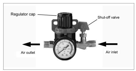
The unit can be isolated from the air supply by screwing down the shut off valve on the inlet side of the unit. To restore airflow, unscrew the valve no more than 3 full turns from the fully closed position.
