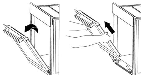
8. Pull the removed door upwards to release it from the right and left hinges and remove it.
