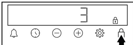
⇒ The 🔒 symbol is shown on the display and the 3-2-1 count down starts. The key lock activates when the countdown ends. When any key is touched after the key lock is set, the timer sounds an audible signal and the 🔒 symbol flashes.
