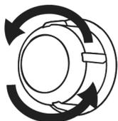
3. If your oven lamp is type (A) shown in the figure below, rotate the oven lamp as shown in the figure and replace it with a new one. If it is type (B) model, pull it out as shown in the figure and replace it with a new one.
