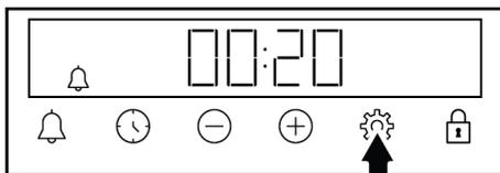
⇒ After setting the alarm time, the 🔔 symbol remains lit and the alarm time starts to countdown on the display. If the alarm time and baking time are set at the same time, the shorter time is shown on the display.
