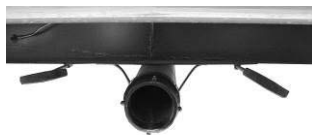
Black/Grey tank drain & valves
