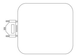
Secure the 15-pin connector onto the Vehicle Gateway using the thumbscrews.
