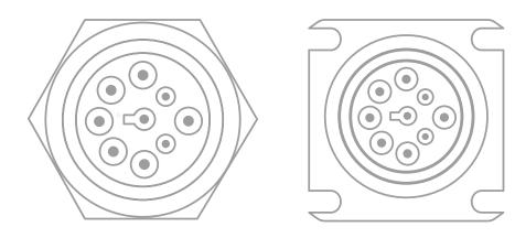
Attach the 9-Pin Y-cable to the vehicle's 9-Pin port and replace the vehicle's exposed 9-Pin port with the matching end of the 9-Pin Y-cable.
