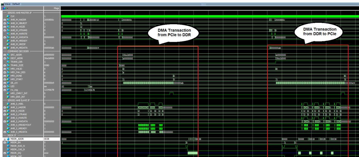
Figure 4 • DMA Transactions between PCIe and LPDDR
