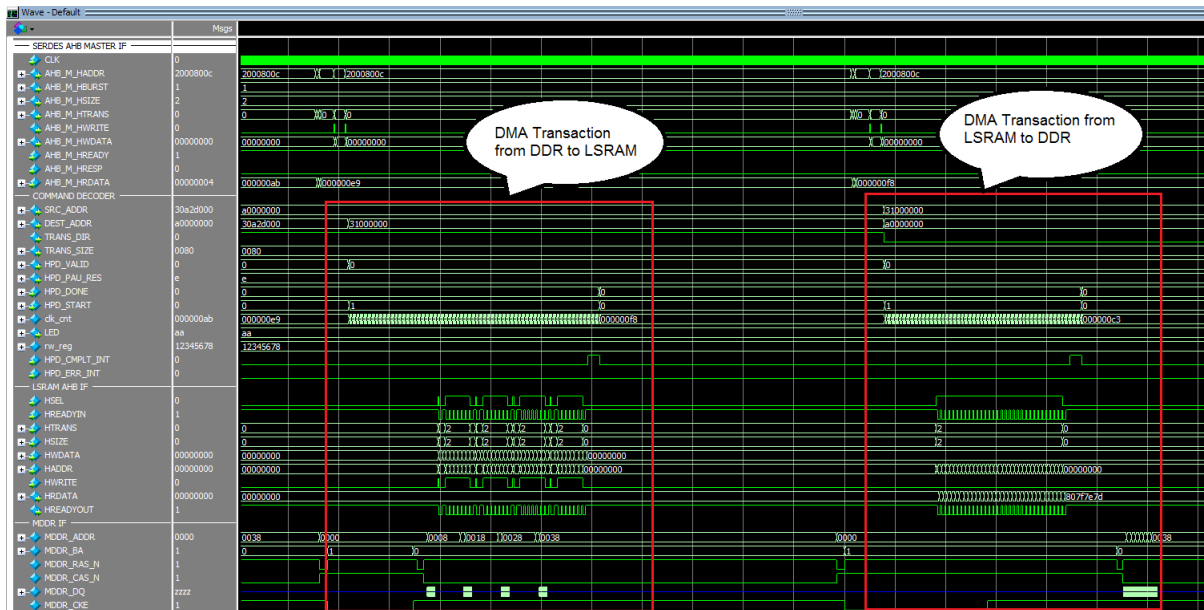
Figure 5 • DMA Transactions between LPDDR and LSRAM
