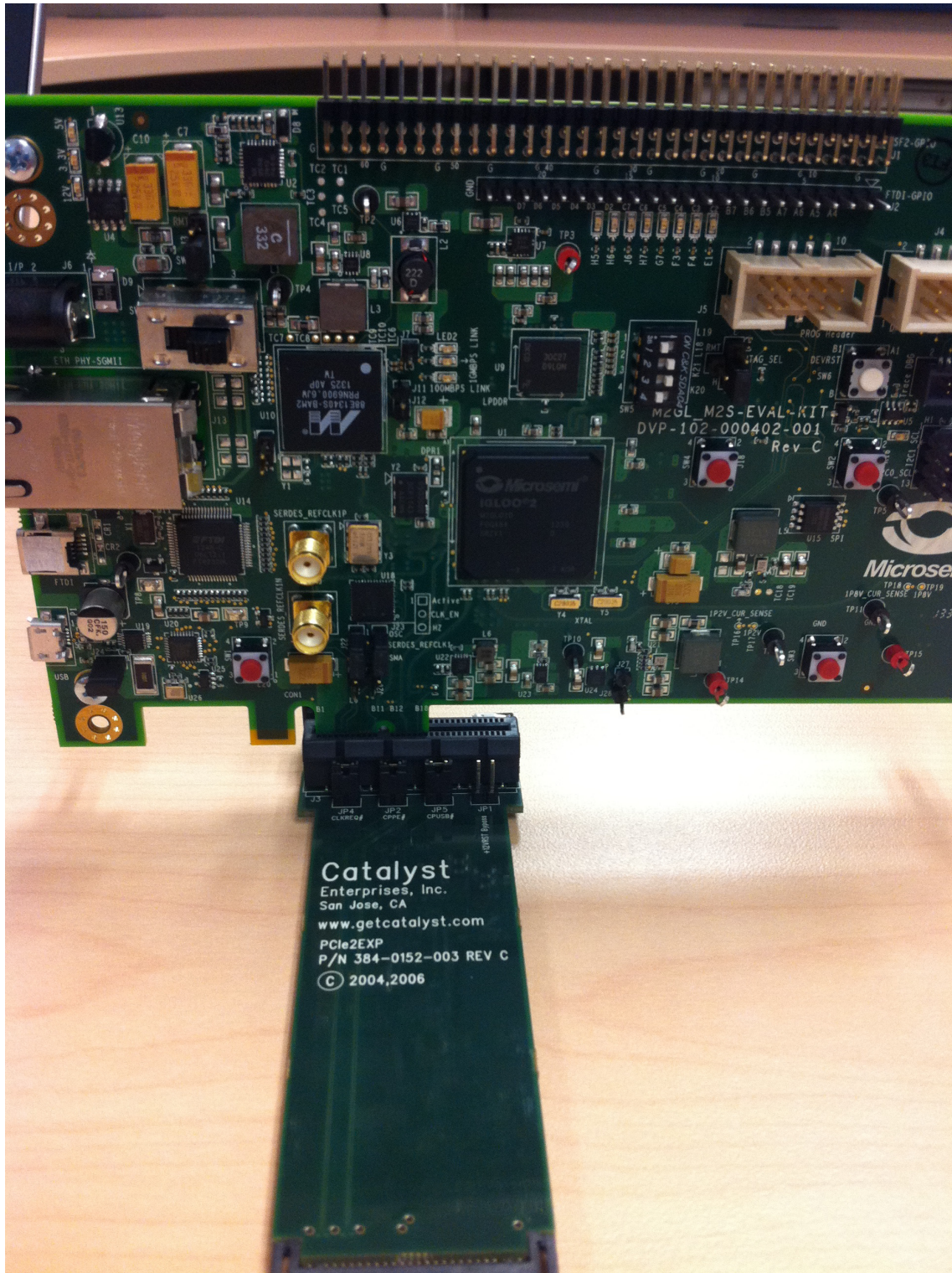
Figure 32 • Inserting the IGLOO2 Evaluation Kit PCIe Connector into the PCIe Adapter Card Slot
