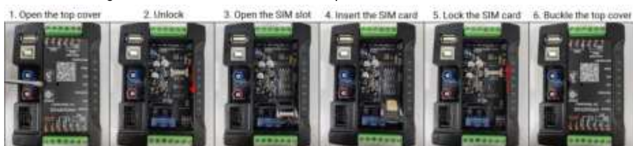
Fig.3 – SIM Card Installation Steps
