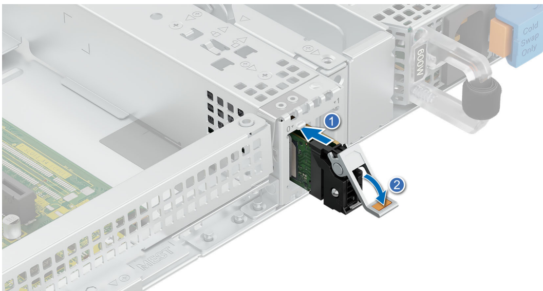
Figure 80. Installing the BOSS-N1 M.2 module
