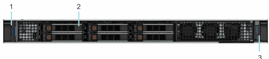
Figure 3. Front view of 6 x 2.5-inch drive system
