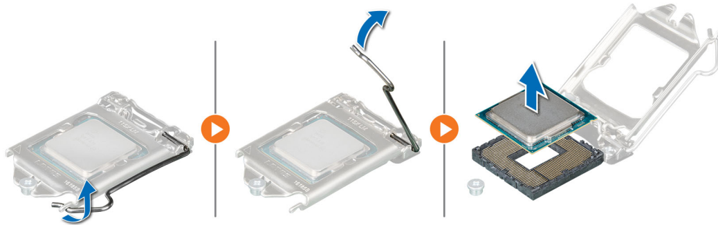
Figure 59. Removing the processor
