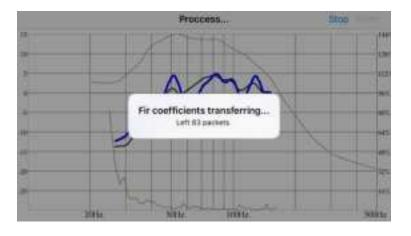
4) The image below shows an example result of a completed correction process. This measurement was completed using the linear mode of correction, and three measurements averaged together for both near field and listening position. The result also used all of the settings found in previous screenshots.
