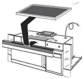
Filter Kit JX81C— Recirculating Charcoal Filter Kit To be used when the Spacemaker microwave oven cannot be vented to the outside.
