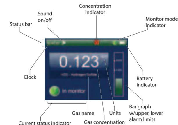
Figure 3: SPM Flex display - In Monitor mode
