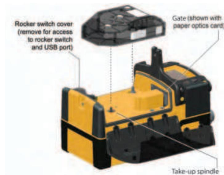
Figure 9: Loading a Chemcassette cartridge
