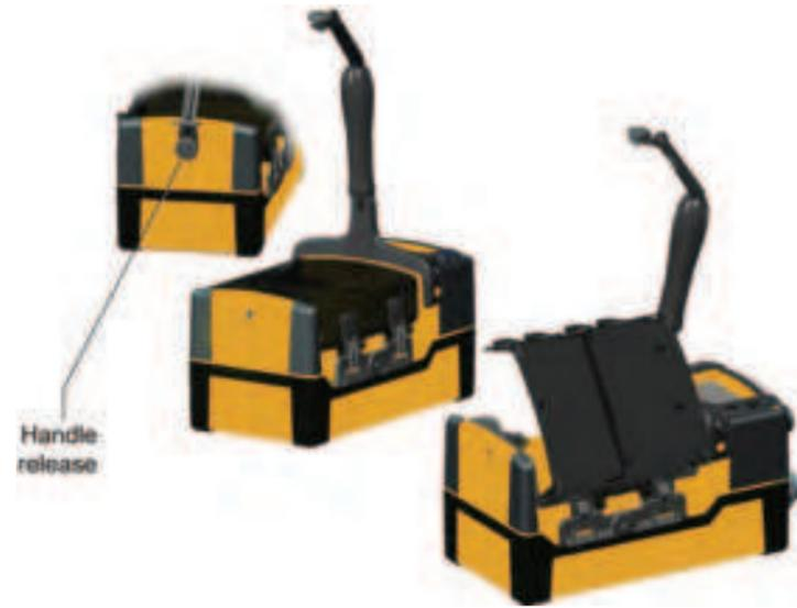
Figure 8: Opening the Chemcassette cartridge door
