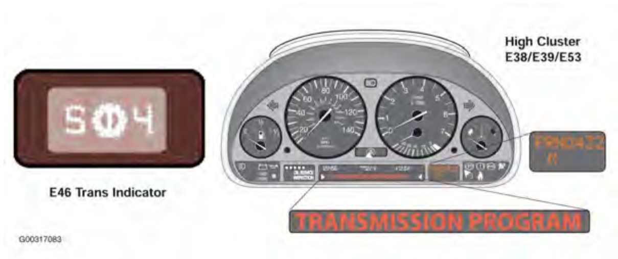
Fig. 24: Identifying Instrument Cluster Transmission Information Courtesy of BMW OF NORTH AMERICA, INC.
