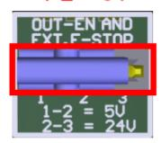
If used a power supply of 24VDC and in the output of terminal de EN and EXT E-STOP wwork with 24V, set jumper as sample in the image.
