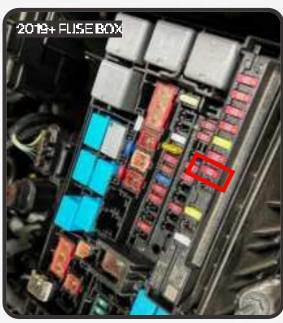
22. INSERT THE FUSE YOU REMOVED FROM THE FUSE BOX INTO THE EMPTY FUSE SLOT OF THE SUPPLIED FUSE TAP HARNESS. THEN, INSERT THE FUSE TAP INTO THE INJECTOR FUSE YOU REMOVED THE
