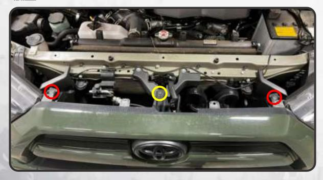
3. FIRMLY PULL THE UPPER GRILLE FORWARD, RELEASING THE GCLIPS SECURING IT, AND REMOVEIT FROM THE VEHICLE
