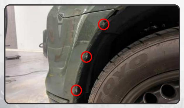
5. REMOVE THE TWO 10MM SCREWS FROM THE UNDERSIDE OF THE BUMPER.
