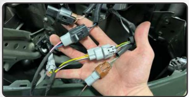
28. IF YOUR VEHICLE CAME EQUIPPED WITH THE LED LOW BEAM AND HALOGEN HIGH BEAM FACTORY HEADLIGHTS, TAKE THE LED ADAPTER HARNESS AND REMOVETHE CAP ON THE BLACK CONNECTOR. THEN, MATCH THE FOUR FACTORY HEADLIGHT CONNECTORS TO THE FOUR CORRESPONDING CONNECTORS ON THE HARNESS, AND THE SINGLE REMAINING CONNECTOR TO THE RESISTOR. REPEAT ON THE OPPOSITE SIDE OF THE VEHICLE
