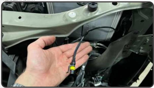
26. ROUTETHE LONG END OF THE HARNESS ACROSS TO THE PASSENGER-SIDE HEADLIGHT CAVITY. WE RECOMMEND ROUTING IT ACROSS THE TOP OF THE RADIATOR SUPPORT AND SECURING IT IN PLACE WITH ZIPTIES. MAKE SURE ANY LOOSE/EXCESS WIRING IS TUCKED AWAY IN A SAFE LOCATION AND SECURED
