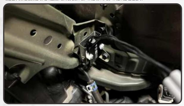
28. IF YOUR VEHICLE CAME EQUIPPED WITH THE FULLY HALOGEN FACTORY HEADLIGHTS, TAKE THE HALOGEN ADAPTER HARNESS AND MATCH THE FOUR CONNECTORS ON IT TO THE FOUR FACTORY HEADLIGHT CONNECTORS ON THE VEHICLE, AND THE SINGLE REMAINING CONNECTOR TO THE RESISTOR. REPEAT ON THE OPPOSITE SIDE OF THE VEHICLE
