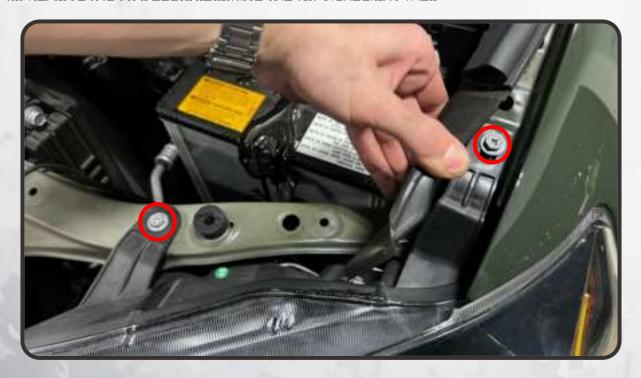
11. LIFT UP ON THOSE TWO UPPER HEADLIGHT TABS AND PULL THE HEADLIGHT FORWARD. FLEX THE BLIMPER COVER OUT OF THE WAY AND PULL THE HEADLIGHT OFF OF THE VEHICLE ENOUGH TO DISCONNECT THE FOUR PLUGS ON THE BACK OF THE LIGHT. WITH THE PLUGS DISCONNECTED, REMOVE THE LIGHT AND SET IT ASIDE
