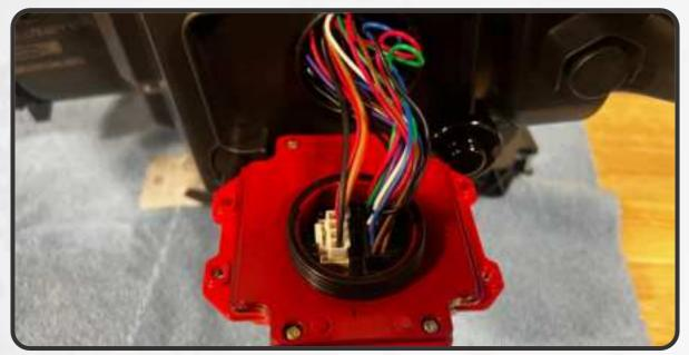
20. APPLY A SMALL AMOUNT OF THE INCLUDED GREASE TO THE SEAL OF THE NEW DRIVER.
