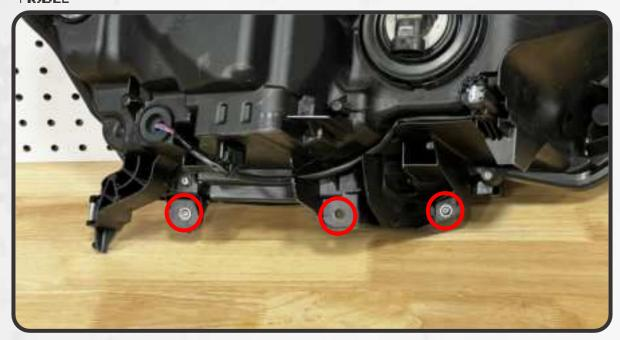
14. TRANSFER THE BRACKET OVER TO THE NEW HEADLIGHT ASSEMBLY, AND SECURE IT USING THE FACTORY HARDWARE. REPEAT THESE STEPS ON THE OTHER HEADLIGHT ASSEMBLY.
