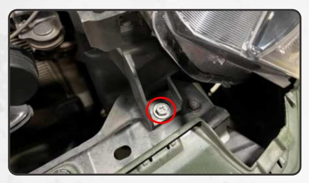
10. REMOVE THE TWO BOLTS SECURING THE TOP HEADLIGHT TABS.
