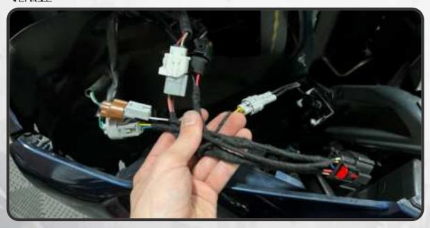
28. IF YOUR VEHICLE CAME EQUIPPED WITH THE FULLY LED FACTORY HEADLIGHTS, TAKE THE LED ADAPTER HARNESS AND MATCH THE FOUR GREY CONNECTORS ON IT TO THE THREE CORRESPONDING FACTORY HEADLIGHT CONNECTORS ON THE VEHICLE AND THE SINGLE CONNECTOR ON THE RESISTOR. THERE SHOULD BE ONE FACTORY HEADLIGHT CONNECTOR LEFT DISCONNECTED. THIS CONNECTOR IS NOT USED, SO INSTALL THE INCLUDED CONNECTOR CAP ONTO IT. REPEAT ON THE OPPOSITE SIDE OF THE VEHICLE
