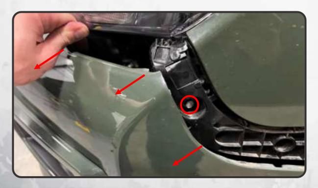
9. REMOVE THE 10MM BOLT ON THE INNER EDGE OF THE HEADLIGHT.
