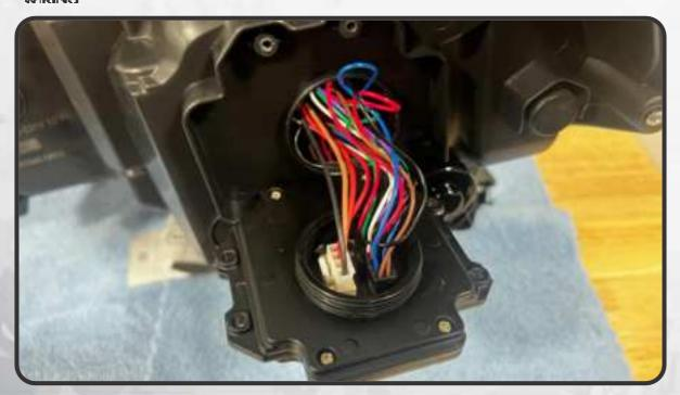
CONNECT THE NEW SUPERCHARGED DRIVER TO THE INTERNAL HEADLIGHT WIRING, MAKING SURE THE TAB ON EACH OF THE CONNECTOR'S CLIPS SECURELY INTO PLACE.
