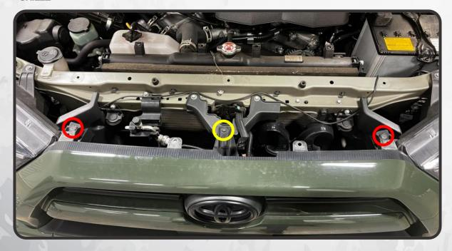
3. FIRMLY PULL THE UPPER GRILLE FORWARD, RELEASING THE 6 CLIPS SECURING IT, AND REMOVE IT FROM THE VEHICLE
