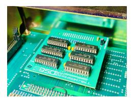
STEP 4 - FIX IT WITH THE PLASTIC WASHER AND M2.5 NUT A plastic washer and M2.5 nut is also included with each RAM module; just tighten it with hand, that should be enough
