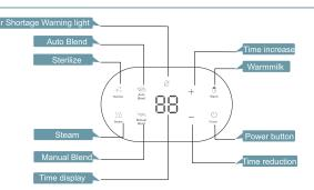
The panel's " $\circlearrowleft$ " indicator goes red when you connect the appliance. It means that the device is ON and ready to use. A white light indicates that the product is button. This button light glows brilliant white when a panel button is pressed. Red light indicates a water shortage warning. The appliance is in standby mode when the time displays " 00 ". In other words, it is functional and ready to use.
