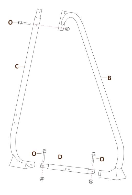
(3). Use **#O** to secure the assembled top bar and triangular support frame.
