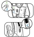
Press the mode switch button to switch to Bluetooth mode until the top blue light flashes slowly and enter Bluetooth mode.
