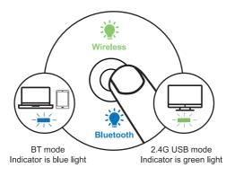
Press the mode switch button at the bottom of the mouse.
