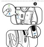
3. Press and hold the mode switch button for 3~5 seconds until the top blue light flashes quickly, then the mouse enters the Bluetooth pairing mode.
