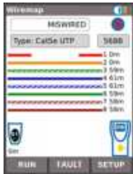
Fig 20 Open circuit by pin
