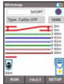
Fig 21 Short circuit by pin
