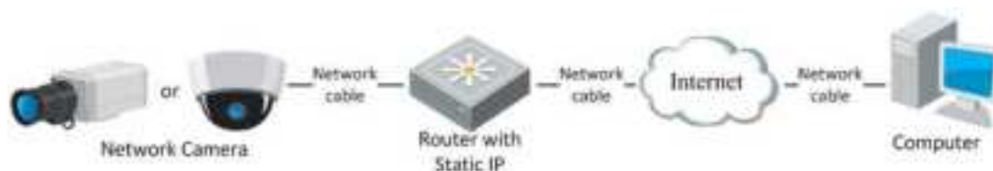
Figure 2-10 Accessing the Camera through Router with Static IP
