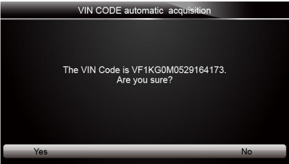
Figure 4-3 Sample VIN Automatic Acquisition
