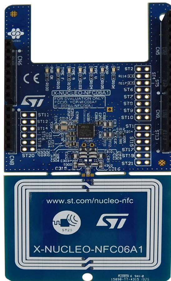
Figure 9. X-NUCLEO-NFC06A1 expansion board
