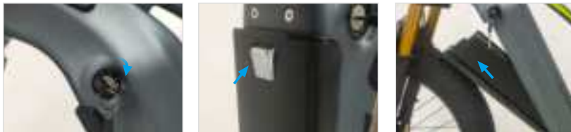
Open the battery lock
