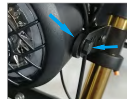
10. As shown, the gasket is installed
