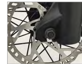
5. Tighten the left and right nuts as shown
