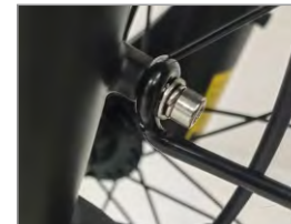
7. Install the fender bracket screws
