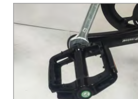
12. Take out the pedal with the letters "R" and "L", align it with the crank hole and lock it with a wrench
