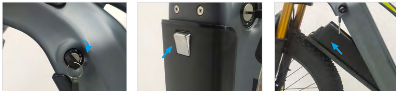
Open the battery lock
