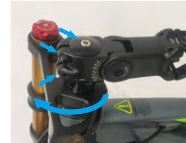
1. Adjust the top and left and right screws to rotate the adjustable riser 180 degrees and secure it in place
