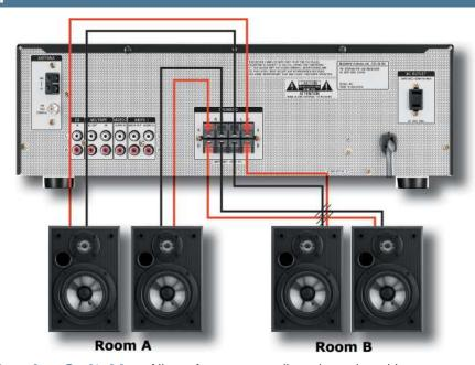
A and B Speaker Switching Allows for stereo audio to be enjoyed in two separate rooms.
